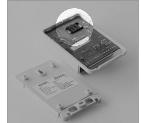
02 • Insert the SIM card (WITH DISABLED PIN) in the SIM's drawer on the back of M150SP.
