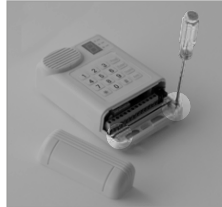
01 • Open the equipment with the help of proper tool and remove the back cover.
