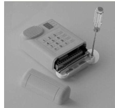
01 • Open the equipment with the help of a proper tool and remove the back cover.
